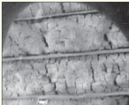
Glowing logs, separated by mineral wool, at 2000°F in the furnace.
